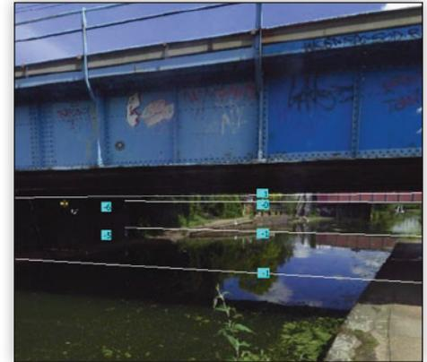
GSDMon is a tool which facilitates the storing, displaying and analysing of monitoring data. Bespoke views show monitoring data overlaid onto site images to provide quick overview of monitoring status.
