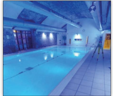
3D Laser scanning has been a fundamental part of the design process for the London Bridge project. In simple terms a laser scanner can take multiple scans from any site quickly – scanning up to one million points of data per second. In the office, the resulting point clouds can be modelled in various software packages such as Microstation, Rhinoceros, Pointools or AutoCad. The result is a highly detailed full-scale 3D model that has many uses for the end user.
