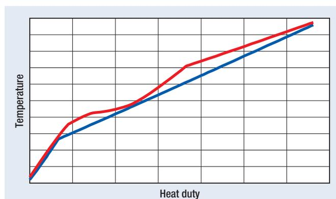
FIG. 3 Typical cooling curves for dual turbo-expander liquefaction.
