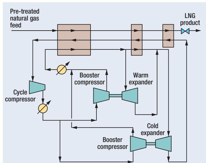
FIG. 2 Dual turbo-expander flowsheet for gas liquefaction.
