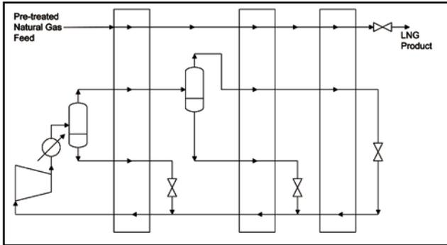
**Figure 4. Typical three stage mixed refrigerant cycle.**
